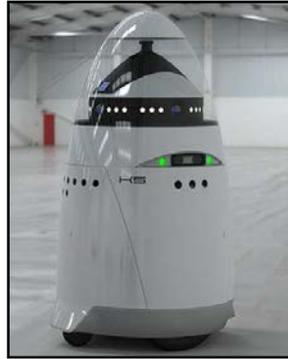
robot can be used to display messages. They are self-monitoring and return to the charging plate when batteries need recharging.
